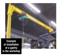
With the VERLINDE range of independent manual-travel gantries, any crew of mounting fitters or a craft mechanic can carry out all maintenance, removal, re-installation and locating operations on parts or assemblies. This range of standard gantries is designed to accommodate any hoist and can be equipped with either or a hand or electric-powered chain hoist.
