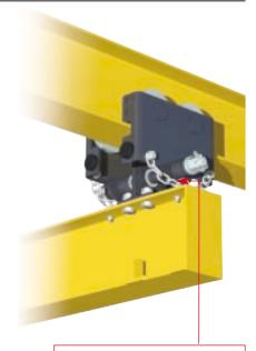
As optional extra: 2 safety chains. The purpose of this system is to restore the link between the trolleys and beam in the event of failure of the coupling linking the trolleys to the beam.
